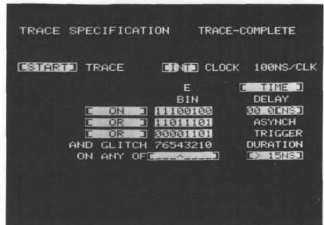
Figure 1. Trace Specifications menu shows the label assigned to the timing lines and the numerical base in which to enter data. This Trace Specification defines the start of data collection using an internal clock running 100 ns/clock on any one of three OR'ed 8-bit patterns but only if a glitch appears on channel four.
