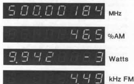
Modulation Analyzer displays of RF signal parameters.
