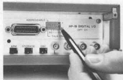
Rear panel switches are set so instrument will either be addressable by controller in a multi-device system, or will simply "talk only" to another device such as a printer.
