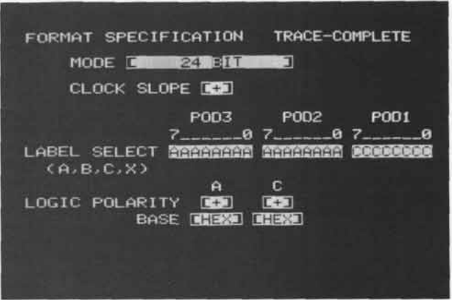
Figure 4. To monitor 24 lines of synchronous activity, a 24 Bit mode of operation may be selected. Labels, Clock Slope, Logic Polarity, and Bases are assigned to obtain the desired Format. This Format is selected to display 16 address lines (Label A) and 8 data lines (Label C) both in hexadecimal.
